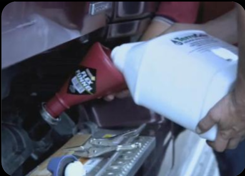
Trucks are filled with liquid urea SCR prior to departing for testing run.
