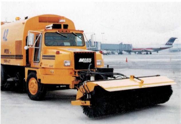
Front mounted snow broom available with some chassis. Consult factory.
