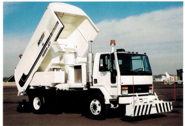
Debris container in dump position. Clean design for easy maintenance.
